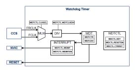
The WDT is a 24-bit count-down timer. This timer may be configured to be clocked either from the FRCLK (input to the PLL) or FCLK (output of the PLL). Because of this, this timer may be used as a wakeup timer when the ARM Cortex-M0 is in deep sleep mode.
